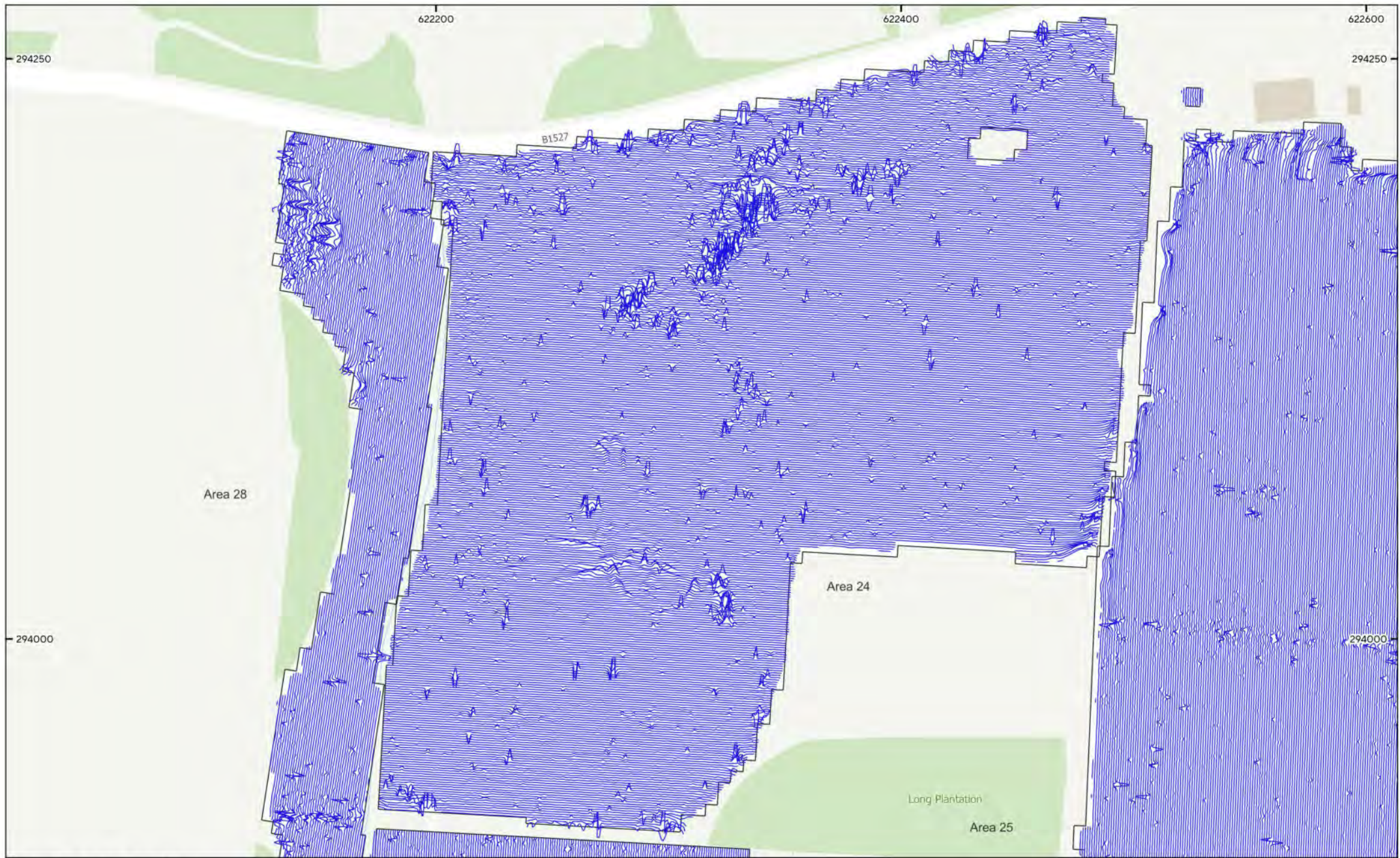
MSTM1774 - East Pye Solar Farm Figure 196 - Area of Archaeological Activity 4 (Areas 24 & 28) XY Trace Plot 90nT/cm at 1:1,500 @ A3 © Magnitude Surveys 2025 Contains Ordnance Survey data © Crown Copyright and database right 2025
