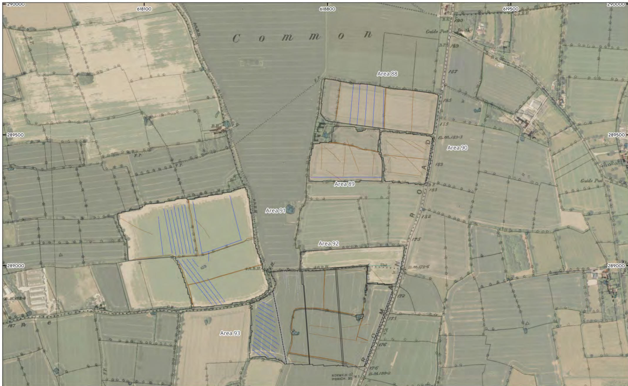
MSTM1774 - East Pye Solar Farm Figure 12 - Magnetic Interpretation over Historical Map and Satellite Imagery (Site 2 (Areas 88 to 93)) 1:6,000 @ A3 © Magnitude Surveys 2025 Contains historical mapping © CLS data Ordnance Survey 6" 2nd edition c.1882-1913 Contains satellite imagery © Bing Satellite 2025
