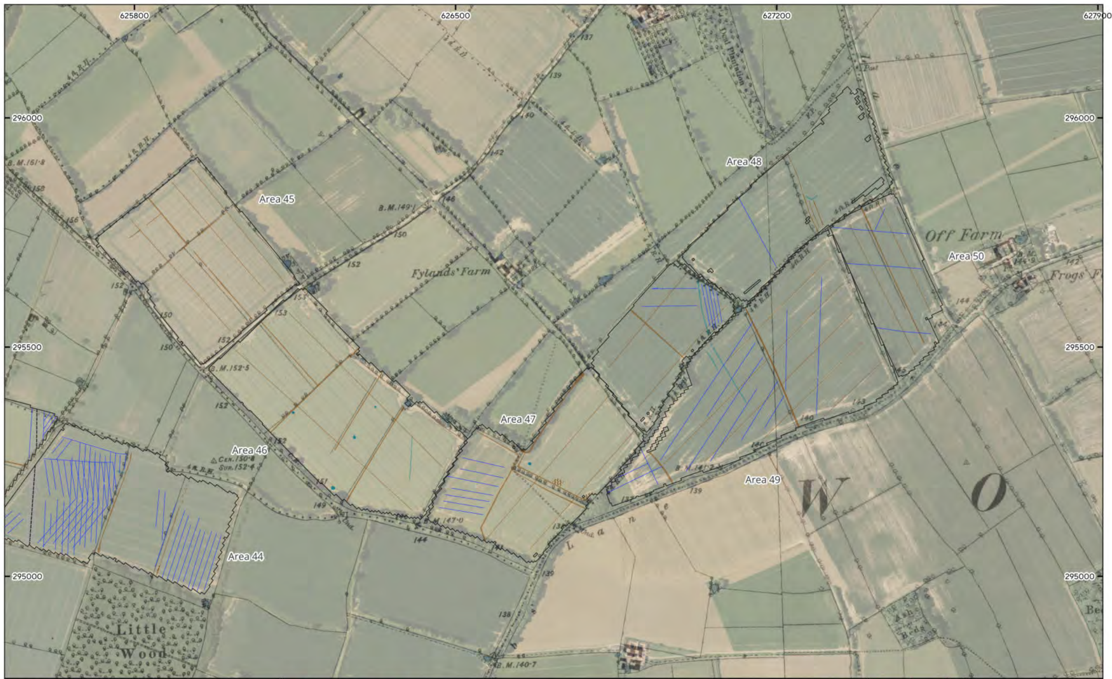
MSTM1774 - East Pye Solar Farm Figure 36 - Magnetic Interpretation over Historical Map and Satellite Imagery (Site 7 (East) (Areas 44 & 45 to 50)) 1:6,000 @ A3 © Magnitude Surveys 2025 Contains historical mapping © CLS data Ordnance Survey 6" 2nd edition c. 1882-1913 Contains satellite imagery © Bing Satellite 2025
