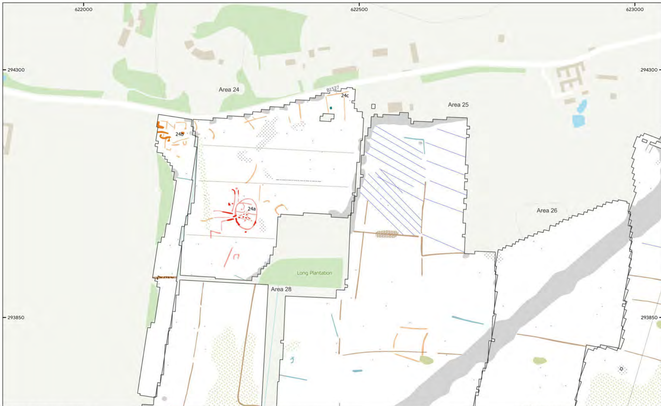
MSTM1774 - East Pye Solar Farm Figure 111 - Magnetic Interpretation (Areas 24 to 26 & 29) 1:3,000 @ A3 © Magnitude Surveys 2025 Contains Ordnance Survey data © Crown Copyright and database right 2025
