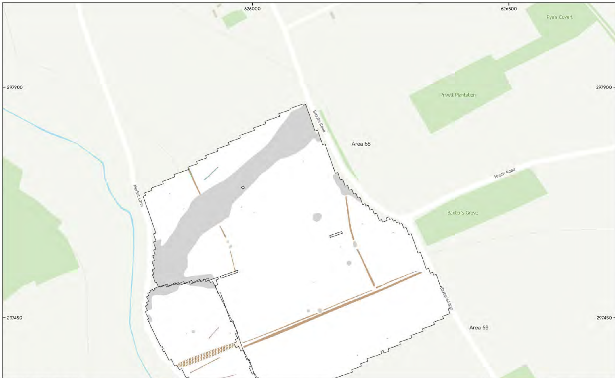
MSTM1774 - East Pye Solar Farm Figure 159 - Magnetic Interpretation (Areas 58 to 60) 1:3,000 @ A3 © Magnitude Surveys 2025 Contains Ordnance Survey data © Crown Copyright and database right 2025
