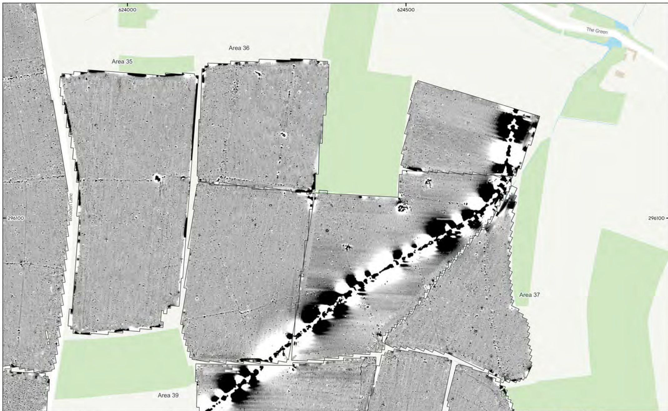
MSTM1774 - East Pye Solar Farm Figure 125 - Magnetic Gradient (Areas 33 to 37 & 39 to 41) 1:3,000 @ A3 © Magnitude Surveys 2025 Contains Ordnance Survey data © Crown Copyright and database right 2025
