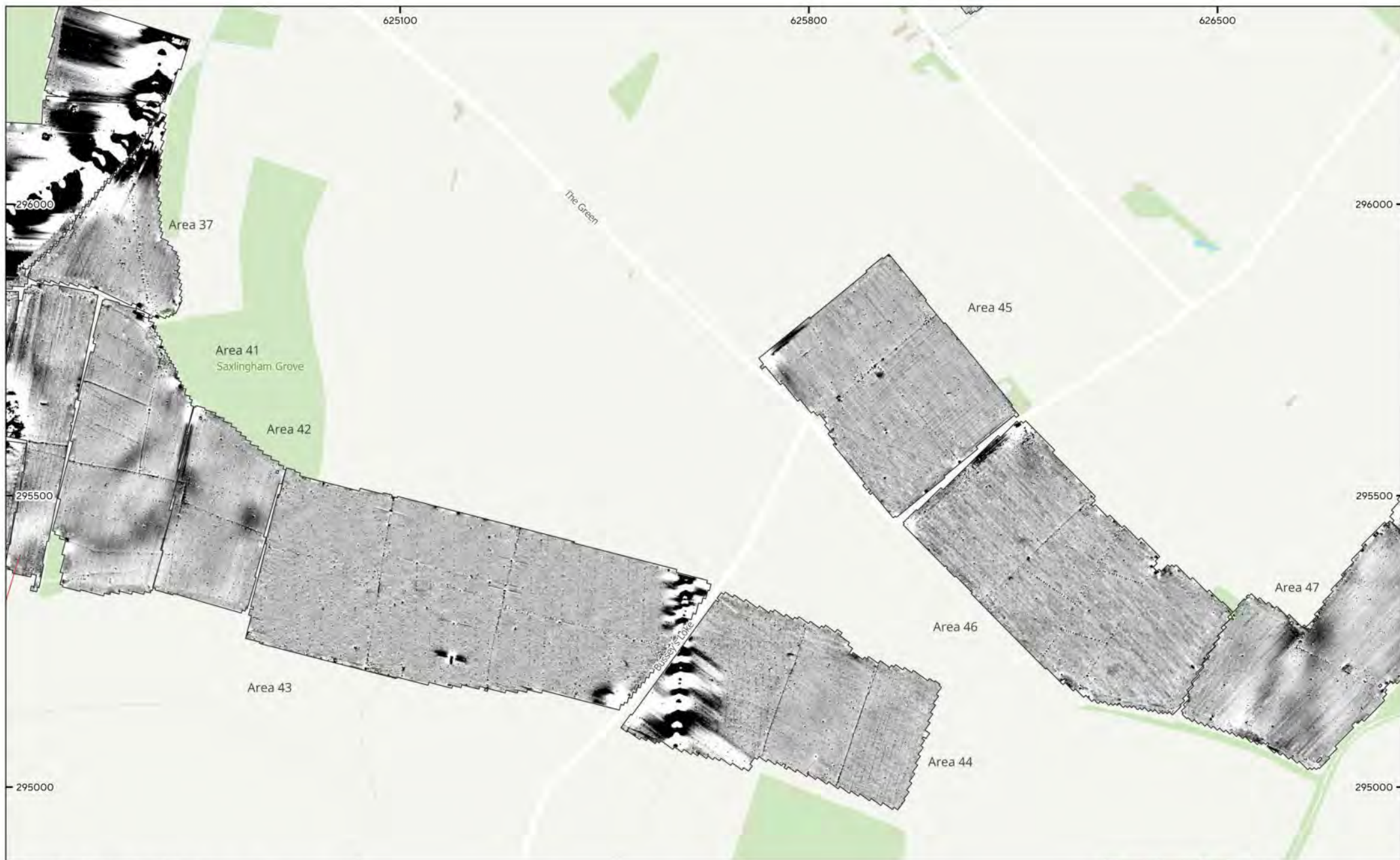
MSTM1774 - East Pye Solar Farm Figure 32 - Magnetic Total Field Overview (Site 7 (Centre) (Areas 36 to 44 & 45 to 47)) 1:6,000 @ A3 © Magnitude Surveys 2025 Contains Ordnance Survey data © Crown Copyright and database right 2025
